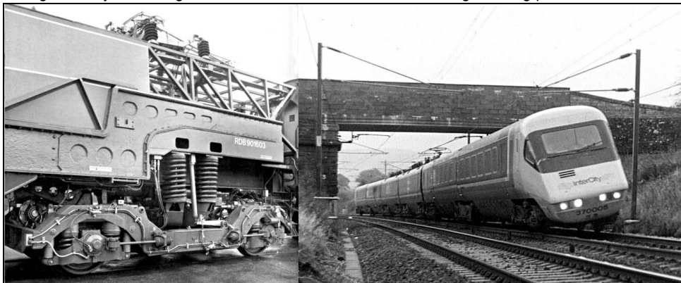
A Trestol wagon rigged with P-Train power bogies, gearbox, tilt and HK brakes to test the pantograph's tilt-compensating mount. Right: This 4+2 formation weighed less than 270 tons. If both power-cars were working its performance would have been quite something.
