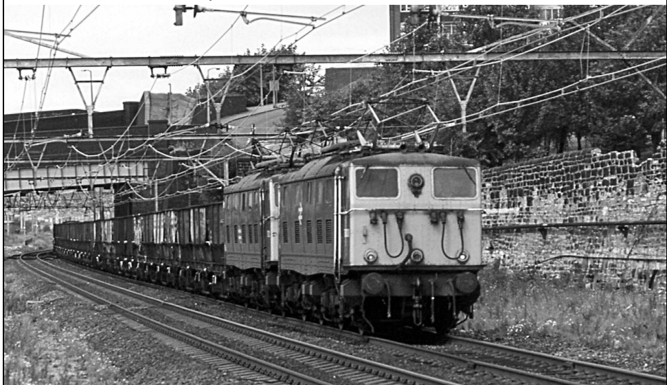
Freight (and Fiddler's Ferry!). 1,500v DC Class 76s bring empty 21ton unfitted coal hoppers past Sheffield in 1980 on the already doomed Woodhead route. NS.
