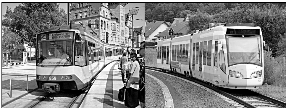
Tram-trains operating in Germany. Street running on the dual voltage Karlsruhe Stadtbahn (left) and a French built Kassel electro-Diesel unit on the main line approaching Wolfhagen on Diesel. Both pictures from Wikipedia used under the terms of the Wikipedia Commons licence.
