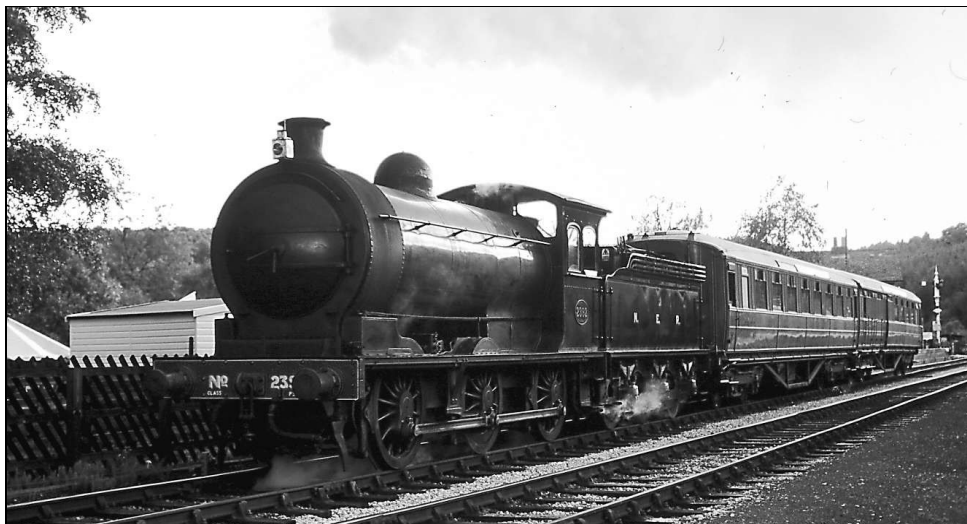
J27 0-6-0 number 2392 is the youngest of her class and the only preserved example. She emerged from Darlington North Road Works in 1923 making her an early LNER locomotive. The fussy might grumble about the NER livery but the LNER built J27s were essentially the last batch of P3s- another enduring Worsdell design. She rests at Levisham with teak coaches.
