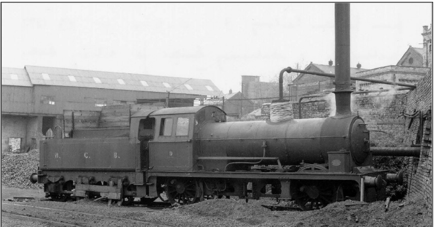
The Works built loco's were much modified throughout their lives especially in N.C.B. ownership. Number 9 ended her long life working as a stationary boiler at Brancepeth Colliery, Willington where she is seen missing her central driving axle, roughly plumbed in and sporting a crude chimney extension. She was cut up here in August 1965.
